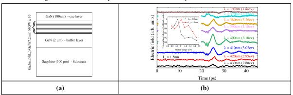
Figure 1. (a) shows the sample schematics, and (b) The wavelength dependence for the MQW sample (inset) shows the comparison between different  $L_z = 1.5$ nm and  $L_z = 3.0$ nm.
