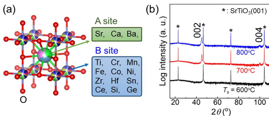
Figure 1. (a) High-entropy ABO<sub>3</sub> perovskite structure and selected elements in A and B sites. (b) Substrate temperature ( $T_s$ ) dependence of out-of-plane X-ray diffraction patterns for the fabricated thin films.
