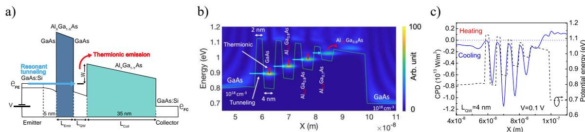
**Figure 1:** a) Schematic representation of the asymmetric double barrier heterostructure [1,2]. b) LDOS (arb. unit) of the quantum cascade cooler (QCC). Horizontal and vertical arrows show the resonant tunneling and thermionic effects respectively. The green solid line represents the potential energy profile; c) Calculated cooling power density (CPD) along the QCC. Negative value corresponding to a cooling phenomenon, the entire QCC is now efficiently refrigerated.
