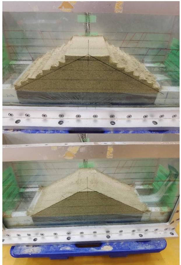
Fig. 4 The model before and after trimming
