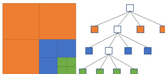
Fig. 1 Tree-type block-structured AMR
