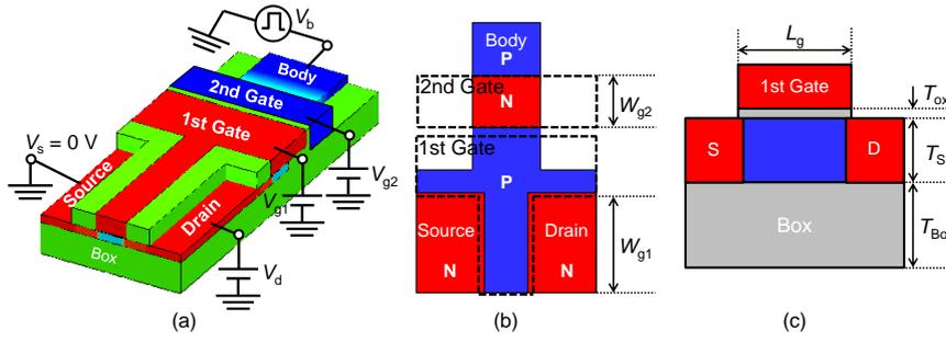
Fig. 1 Device structure of the PNBT SOI-FET. (a) Top-down view. (b) Top view. (c) Front view.
