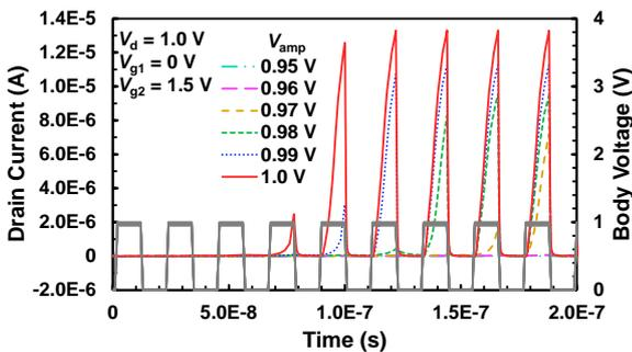
Fig. 6  $I_d$  dependence on pulse amplitude.
