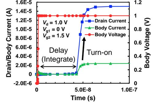
Fig. 3 Transient (turn-on) characteristics of DG PNBT SOI-FET.
