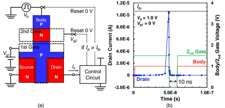
Fig. 7 Spike generation with reset action. (a) Reset circuit. (b)  $I_d$  dependence on time with reset action.
