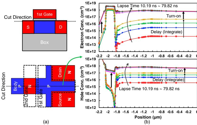
Fig. 4 State of carrier integration. (a) Cut direction. (b) Carrier concentration between integrate and turn-on.
