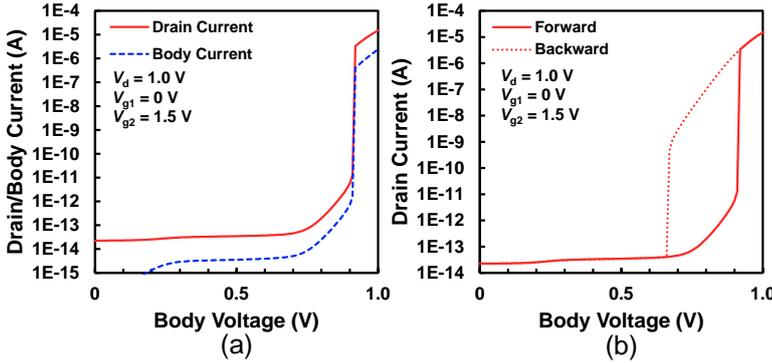
Fig. 2 DC characteristics of DG PNBT SOI-FET. (a)  $I_d$ ,  $I_b$ - $V_b$  characteristics, (b) double sweep characteristics.
