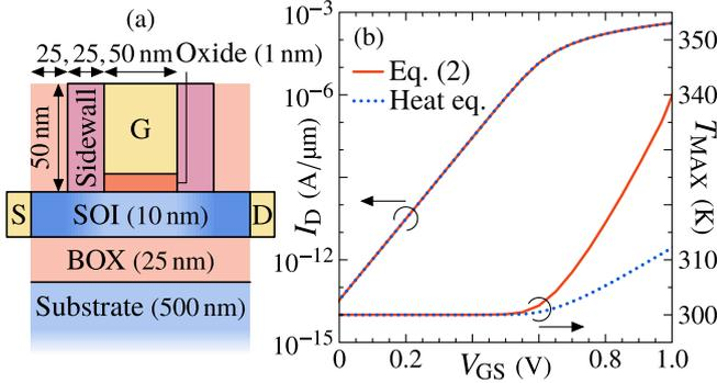
**Fig. 2.** (a) Schematic of a transistor with an SOI body. (b) Its drain current and maximum temperature in the body as functions of the gate-to-source voltage  $V_{GS}$  calculated with (solid lines) or without (dotted lines) taking into account the phonon transport in the body. The drain-to-source voltage was set to 1 V.
