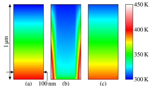
**Fig. 1.** Temperature distributions in a cross-section of Si square bars calculated from (a) the heat equation and [(b) and (c)] the Boltzmann equation of Eq. (2). Only in (c), a boundary condition that phonons are purely specularly reflected was explicitly applied to the bar sides.
