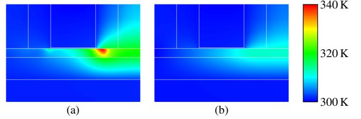
**Fig. 3.** Temperature distributions in the SOI transistor at a  $V_{GS}$  of 1 V simulated (a) with and (b) without taking into account the phonon transport in the SOI body.
