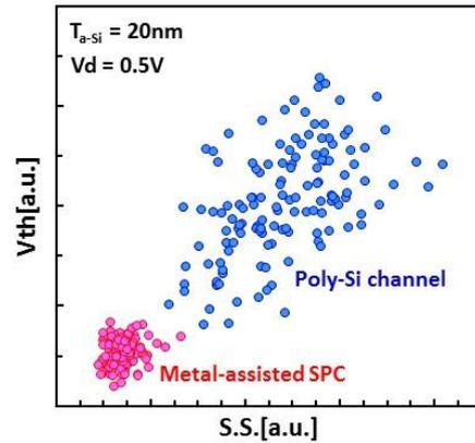
Fig. 5 Correlation between sub-threshold slope (S.S.) and  $V_{th}$  for poly-Si channel and metal-assisted SPC channel (Ref. 4, @2019 IEEE).
