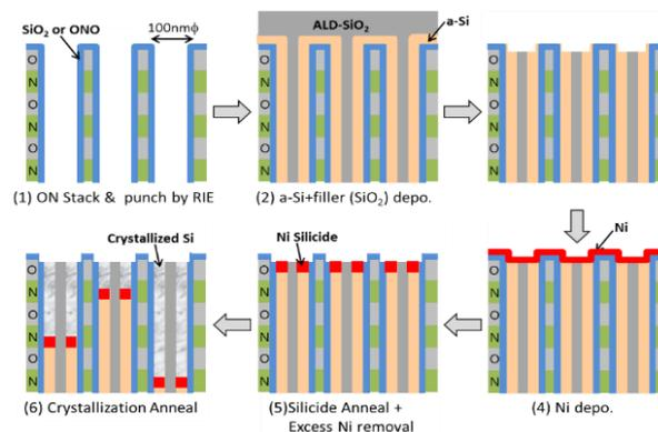
Fig. 1 Application of metal-assisted solid-phase crystallization for vertical holes (Ref. 4, @2019 IEEE).
