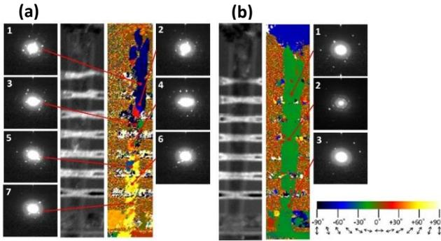
Fig. 3 NBD-2DI images for crystallinity obtained from diffraction patterns, (a) poly Si channel, and (b) metal-assisted SPC Si channel (Ref. 4, @2019 IEEE). The intensity in each position represents the intensity of center beam in each NBD pattern. NBD pattern for each point are also shown. In the color map, the angle of the diffraction spot is measured and displayed for each point in the NBD mapping. The reference angle is set to 0° in the [001] direction of the Si substrate.
