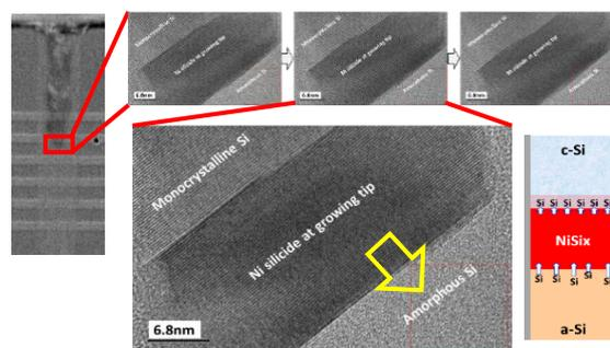
Fig. 2 Snap shots of in-situ TEM image of growing tip for metal-assisted SPC (Ref. 4, @2019 IEEE). It was observed that the epitaxial Ni silicide moves toward amorphous Si and the monocrystalline Si follows.
