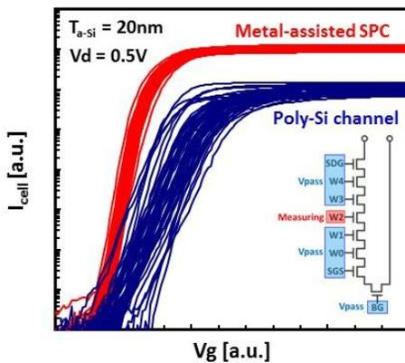
Fig. 4  $V_G$ - $I_{cell}$  characteristics for poly-Si channel, and metal-assisted SPC channel (Ref. 4, @2019 IEEE).
