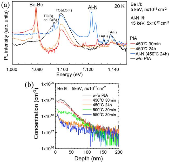
Fig. 2. (a) PL spectra of the energy. Be-Be isoelectronic emission peaks at different PIA times are shown. (b) Impurity depth profiles measured by SIMS for Be.
