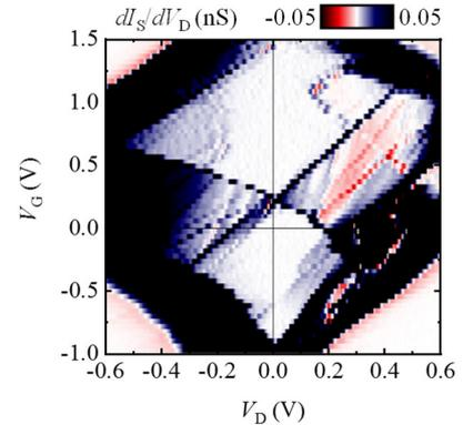
Fig. 4 Linear-scale  $dI_S/dV_D$  maps of a Be-implanted TFET ( $L_g = 80 \text{ nm}$ ,  $W_g = 1 \mu\text{m}$ ) at low temperature (1.5 K).
