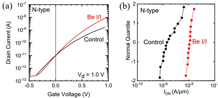
Fig. 3 (a)  $I_D - V_G$  curves of the control and Be implanted IET-TFETs. Their  $L_g$  and  $W_g$  were  $3 \mu\text{m}$  and  $5 \mu\text{m}$ , respectively. (b) Normal quantile plot of  $I_{ON}$ , which was extracted at the voltage of  $V_G - V_{TH} = 1.0 \text{ V}$  with  $V_D = 1.0 \text{ V}$ .
