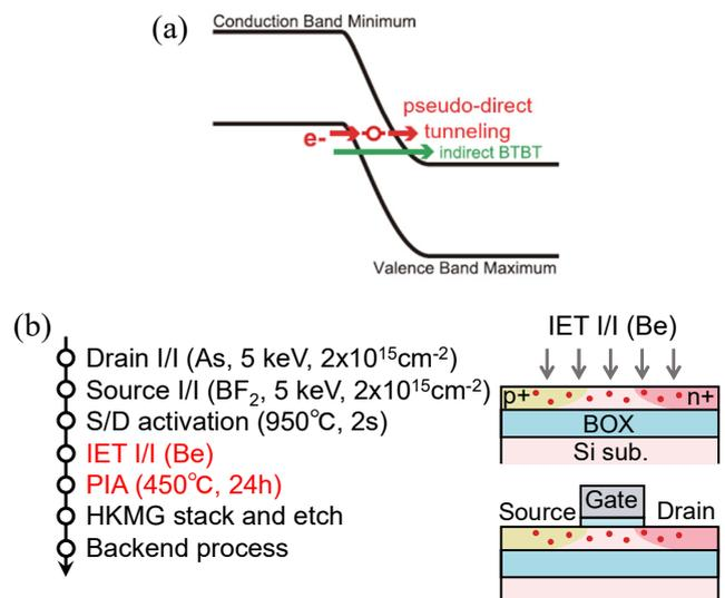
Fig. 1 (a) Schematic of the band diagram of tunneling transport through PN junction. IET intermediated and conventional tunneling paths (indirect BTBT) are illustrated. (b) Process flow and schematic cross-sections of the device fabrication method.
