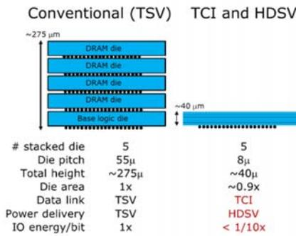
Fig. 7 DRAM stacking with TCI & HDSV.
