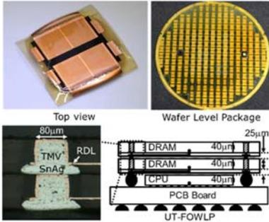
Fig. 4 Ultra-Thin Fan-Out Wafer Level Package.
