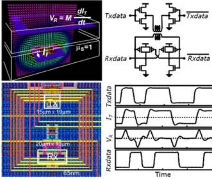
Fig. 1 ThruChip Interface (TCI).
