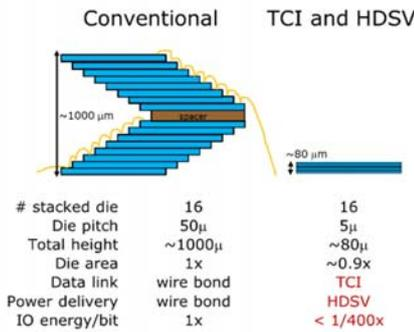
Fig. 6 NAND stacking with TCI & HDSV.
