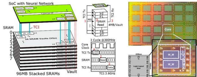
Fig. 5 DNN Inference Engine with Stacked SRAM.
