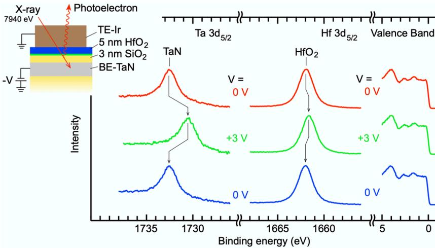
Fig. 6 *In situ* HAXPES measurement of  $\text{Ir}/\text{HfO}_2/1\text{-ML TiO}_2/\text{SiO}_2/\text{TaN}$  MIM stack under bias conditions.
