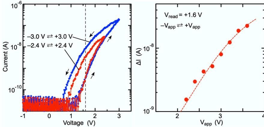
Fig. 3  $I$ - $V$  curves of  $\text{HfO}_2/\text{SiO}_2/\text{HfO}_2$  IDM MIM stack for different bias sweep widths.
