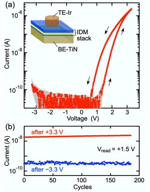
Fig. 2 Current change and rectification characteristics of  $\text{HfO}_2/\text{SiO}_2/\text{HfO}_2$  IDM MIM stack. (a) Cyclic  $I$ - $V$  curves and (b) SET and RESET currents at +1.5 V.
