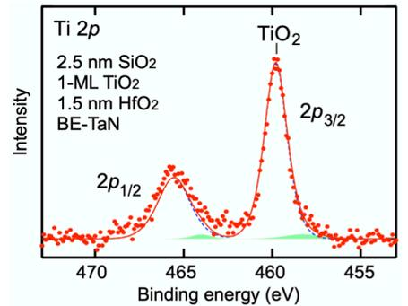
Fig. 5  $\text{Ti } 2p$  photoelectron spectrum of  $\text{SiO}_2/1\text{-ML TiO}_2/\text{HfO}_2$  stack on  $\text{TaN}$  electrode.
