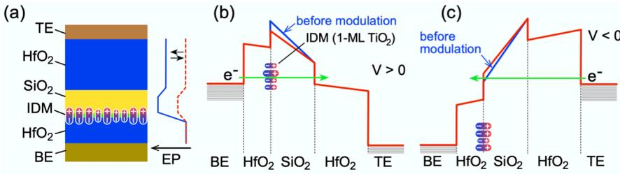
Fig. 1 Concept of rectifying resistive switching MIM stack based on IDM and asymmetric tunnel barrier. (a)  $\text{HfO}_2/\text{SiO}_2/\text{HfO}_2$  MIM stack with 1-ML  $\text{TiO}_2$  modulation layer, (b) and (c) electron barrier height change under positive and negative bias conditions, respectively.
