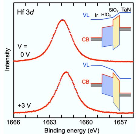
Fig. 7  $\text{Hf } 3d$  photoelectron spectra and predicted band diagrams.
