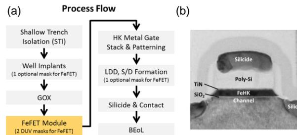
Fig. 1 (a) Schematics of the FeFET technology process flow. (b) TEM cross-section of an embedded FeFET with 9nm thick FeHK HfO<sub>2</sub>.
