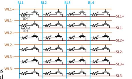
Fig. 7 The schematic diagram of a NOR-type differential ReRAM CIM array.
