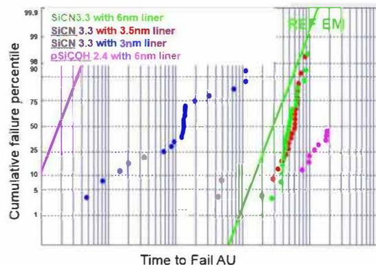
Figure 5. Electromigration performance of sub-50 pitch Cu-Low k SiCN with reference 6nm and thinner liner. Best EM is obtained with thinner 0.6x standard liner/barrier with lower resistance and better TDDB than the reference pSiCOH k=2.45 with 6 nm liner.
