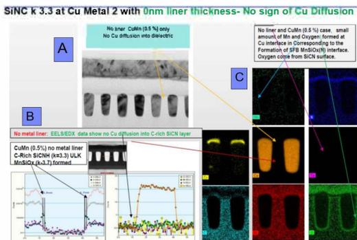
Figure 1. (A) STEM of BEOL M2 Low k C-Rich SiCN-CuMn with no metal liner. (B) SIMS study show no Cu diffusion into C-Rich SiCN and MnSiOx at interfaces. (C) EDX confirms no Cu diffusion or significant PID.
