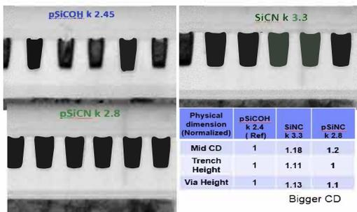
Figure 2. Typical sub-50 nm pitch STEM view and CD of post CMP of Cu-SiCN, pSiCN and pSiCOH 2.4 .
