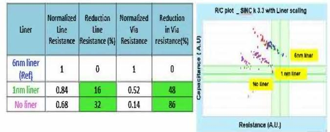
Figure 3. RC Reduction with no and reduced thickness metal liner : measured results for sub-50nm pitch Cu-Low k SiCN BEOL M2 structure.
