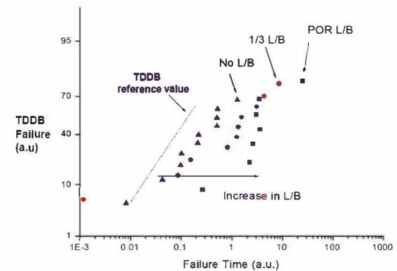
Figure 4- Robust Cu Diffusion and Oxidation barrier properties of SiCN improves sub-50 nm pitch TDDB of CuMn-SiCN even at thinner liner/barrier (L/B).
