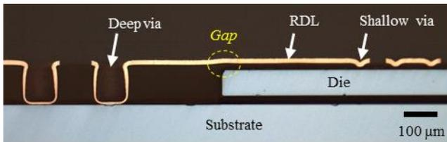
Fig. 3 Cross sections of the embedded die edge.
