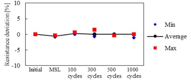
Fig. 5 Resistance deviation during thermal cycle test.
