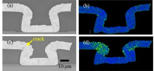
Fig. 4 SEM image and GROD maps of shallow via. (a, b) initial, (c, d) after 1000 thermal cycles.
