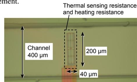
Fig. 3: Close-up image of the thermal sensing resistance and heating resistance under the micro-channel.
