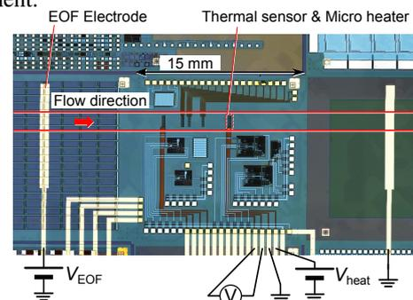
Fig. 2: Photomicrograph of the fabricated on-chip for cooling measurement.
