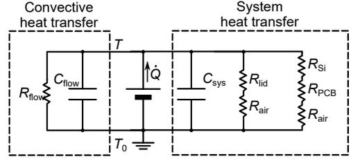
Fig. 6: Schematic of thermal equivalent circuits of the micro-channel cooling system.
