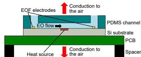
Fig. 1: Schematic of the micro-channel cooling system in the experiment.
