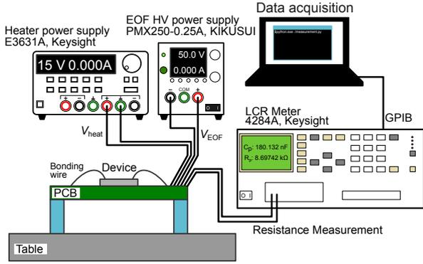
Fig. 4: Schematic view of the experimental setup used for cooling measurement.
