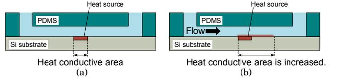
Fig. 7: Conduction heat transfer through silicon substrate (a) without flow and (b) with flow generated by an EOF micropump. When the EOF micropump is turned on, the thermal resistance of the silicon substrate is improved.
