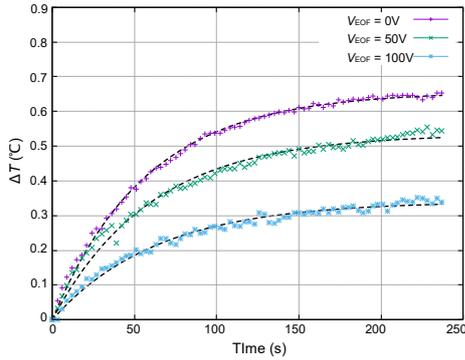
Fig. 5: Measurement result of the change of temperature. At  $t = 0$ , the power is supplied to the microheater.
