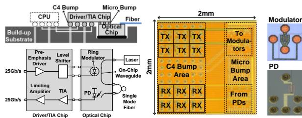
Fig. 6 Transceiver structure, block diagram, chip micrograph
