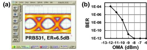
Fig. 8 (a) 25Gb/s TX optical output, (b) RX sensitivity
