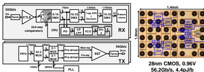
Fig. 2 56Gb/s transceiver block diagram and chip micrograph
