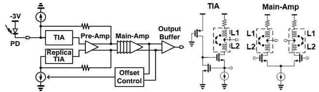
Fig. 7 RX schematic for SiPh transceiver
