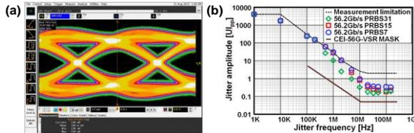
Fig. 5 (a) TX eye diagram (PRBS15), (b) RX jitter tolerance
