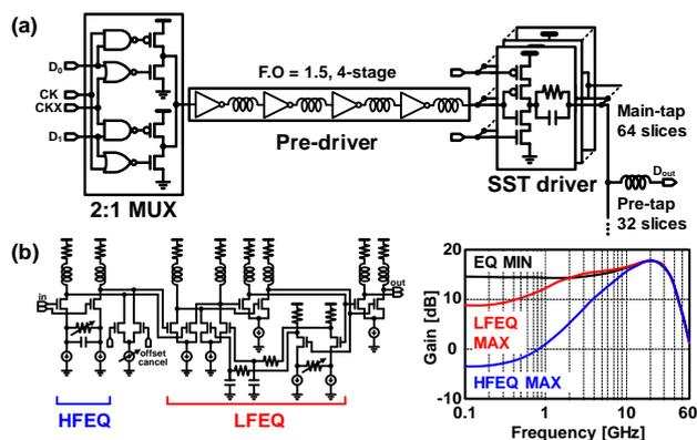
Fig. 3 (a) TX 2-to-1 MUX and SST driver stage, (b) RX CTLE
