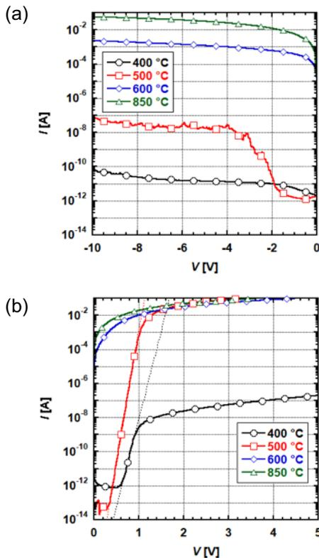
Fig. 2 (a) Reverse and (b) forward  $I$ - $V$  characteristics of the printed Ni Schottky contacts with different  $T_a$  up to 850 °C.
