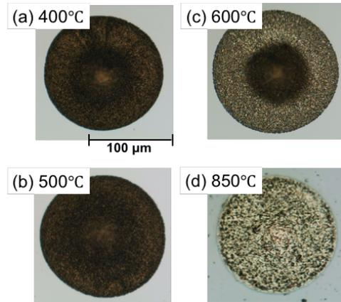
Fig. 4 Optical microscope images of the printed Ni Schottky contacts annealed at (a) 400, (b) 500, (c) 600, and (d) 850 °C.
