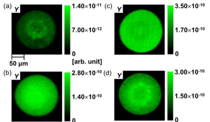
Fig. 5 SIPM  $Y$  maps at  $\lambda = 517$  nm of the Ni Schottky contacts annealed at (a) 400, (b) 500, (c) 600, and (d) 850 °C.
