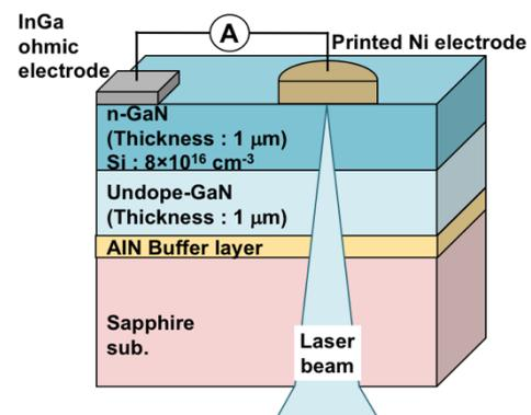
Fig. 1 Printed Ni Schottky contacts formed on the n-GaN epitaxial layer grown on a sapphire substrate by MOCVD.
