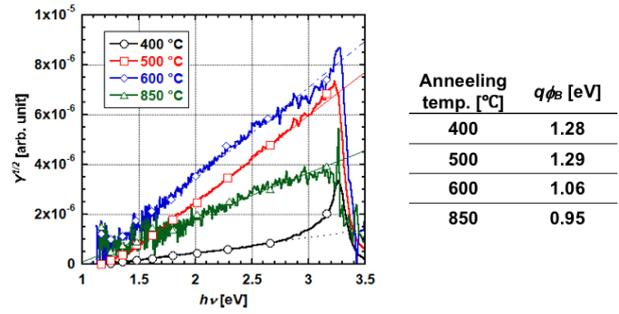
Fig. 3 PR spectra of the printed Ni Schottky contacts annealed up to 850 °C.
