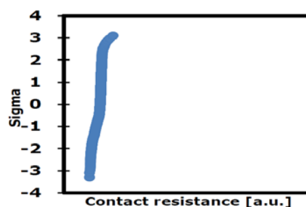
Fig. 3. Cumulative plot of contact resistance of each TSV
