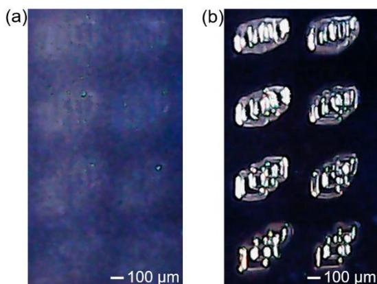
Fig. 3 3D printed microscale structures. (a) Before washing. (b) After washing.
