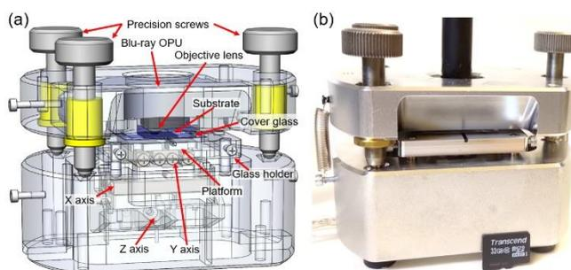
Fig. 1 The BDOPU 3D printing system. (a) a schematic diagram of the system. (b) a photo of the system.
