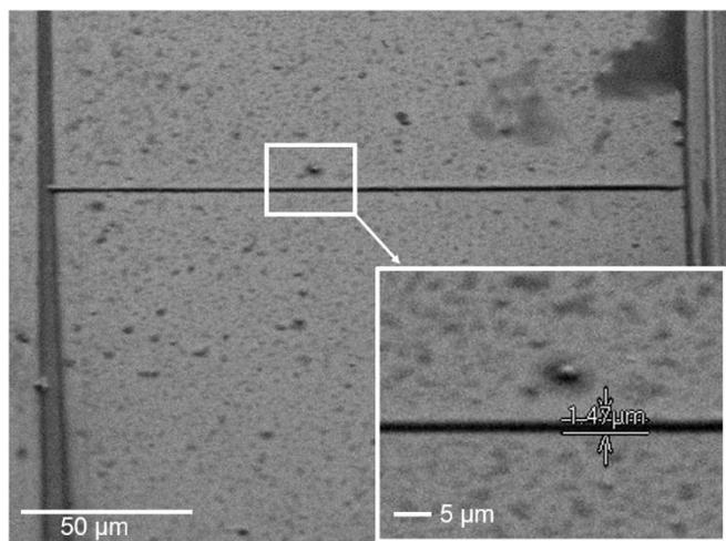
Fig. 4 SEM images of the ladder structure (200x1400  $\mu\text{m}$ ). A zoom-in image shows a line width of 1.47  $\mu\text{m}$ .
