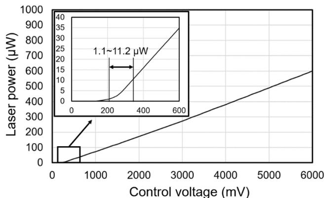
Fig. 2 The BDOPU laser power vs. control voltage. A zoom-in plot shows that the BDOPU 3D printing laser power is between 1.1 and 11.2  $\mu\text{W}$ .
