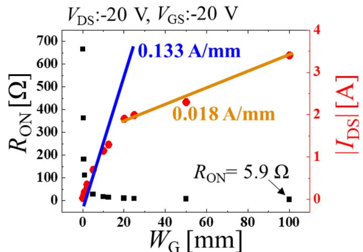
Fig.5 Relationship between drain current ( $|I_{DS}|$ ) and on-resistance ( $R_{ON}$ ) as a function of gate width ( $W_G$ ) at  $V_{DS} = -20$  V and  $V_{GS} = -20$  V.  $R_{ON}$  is 5.9  $\Omega$  when the gate width is 100mm. The current increase amount of 0.133 A/mm is from 0.125 to 20 mm and that of 0.018 A/mm is from 20 to 100 mm. It was caused by source electrode resistance and substrate resistance.
