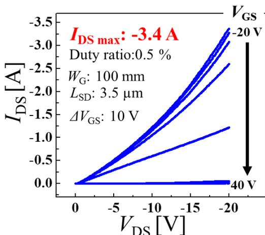
Fig.3  $I_{DS}$ - $V_{DS}$  characteristics using pulse I-V measurement. Duty ratio was 0.5 %. The maximum drain current was  $I_{DS} = -3.4$  A at  $V_{DS} = -20$  V and  $V_{GS} = -20$  V. ( $W_G = 100$  mm,  $L_{SD} = 3.5$   $\mu\text{m}$ ,  $L_G = 2$   $\mu\text{m}$ )
