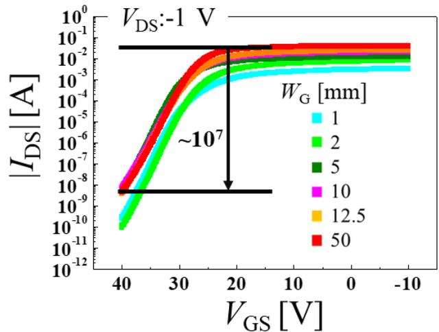
Fig.4  $|I_{DS}|$ - $V_{GS}$  characteristics of 1 mm to 50 mm gate width at  $V_{DS} = -1$  V. On/off ratio is about 7 orders of magnitude for all dimensions. The threshold voltage ( $V_{th}$ ) of these devices was approximately 30 V.
