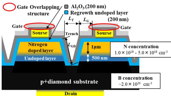
Fig.1 Cross sectional image of vertical-type diamond MOSFETs.  $L_{GD}$  is the drift region on the side wall of the trench.  $L_{SG}$  can be removed because it uses a gate overlapping structure.
