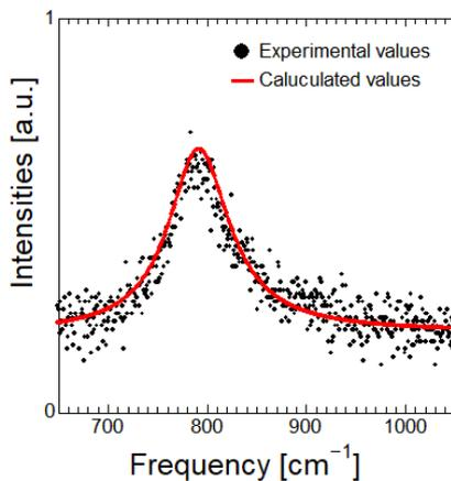
Fig. 3 Comparison of the calculated spectrum for the LOPC mode and experimental spectra at room temperature.
