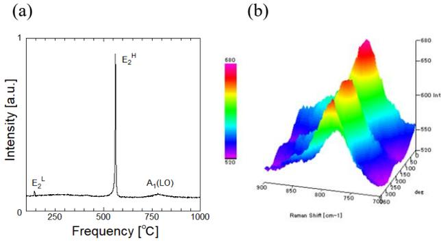
Fig. 1 (a) Raman spectra observed at room temperature and (b) polarized LOPC mode Raman spectra with polarized angles from  $0^\circ$  to  $360^\circ$ .
