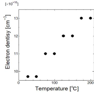
Fig. 4 Temperature dependence of electron density in GaN.
