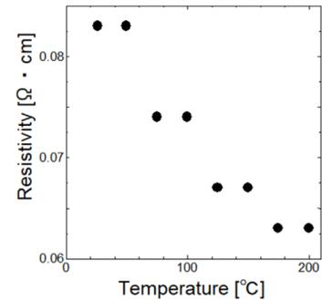
Fig. 5 Temperature dependence of resistivity in GaN.
