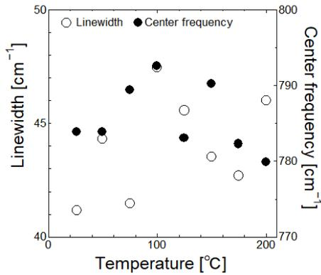
Fig. 2 Temperature dependence of center frequency and linewidth for the LOPC mode of n-type GaN crystals.
