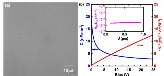
Fig. 1. (a) Cathodoluminescence image of the GaN drift layer and the threading dislocation density is calculated to be 7.4 $\times$ 10<sup>5</sup> cm<sup>-2</sup>. (b) C-V curve of the GaN-on-GaN wafer measured with mercury probe at 10 kHz and inset of (b) extracted depth dependent net doping concentration in the n<sup>-</sup>GaN drift region.
