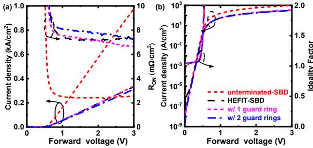
Fig. 3 IV curves of various SBDs with  $d=48 \mu\text{m}$  in (a) linear scale and (b) semi-log scale. The specific on-resistance and ideality factor of SBDs are also shown in the figure.
