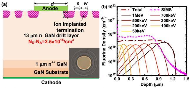
Fig. 2. (a) The schematic cross section view and surface image of the vertical GaN SBD with ion implanted two guard rings. (b) The distribution of F ions from TRIM simulation and the SIMS measurement.
