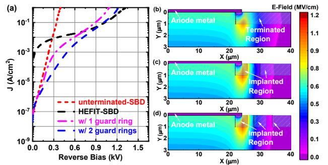
Fig. 4 (a) Reverse characteristics of SBDs. Simulated electric field distribution of the (b) HEFIT-SBD, SBD with (c) one guard ring and (d) two guard rings at  $-400 \text{ V}$ .
