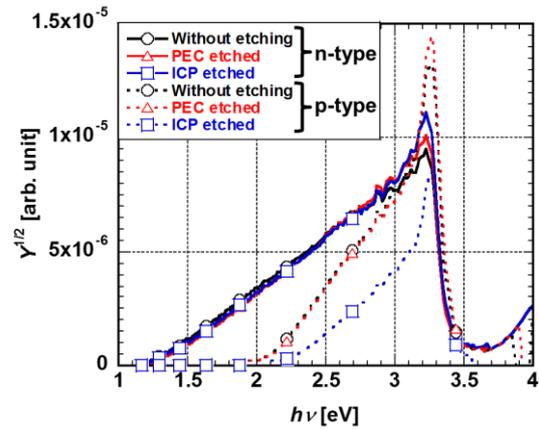
Fig. 3 PR spectra of the n- and p-GaN contacts by PEC or ICP etching.
