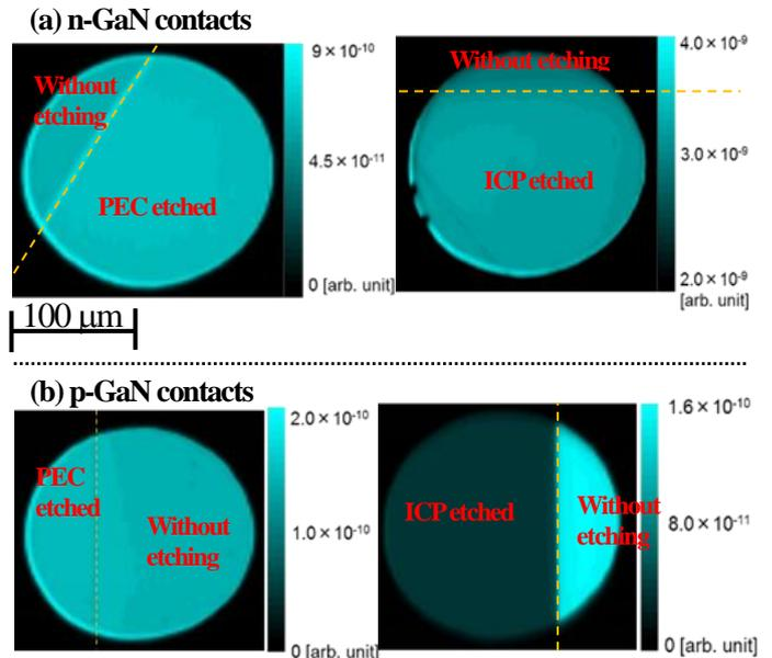
Fig. 4  $Y$  maps ( $\lambda = 447$  nm) of the (a) Ni/n-GaN, and (b) Ni/p-GaN contacts with partially etched regions by PEC or ICP etching.
