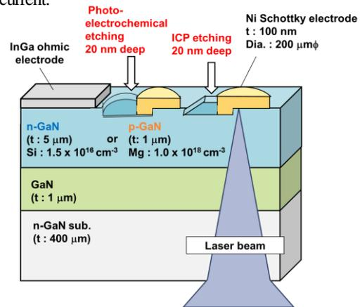
Fig. 1 Device structure. Ni Schottky electrodes were formed on the n-type or p-type GaN surfaces including selectively PEC or ICP etched regions.
