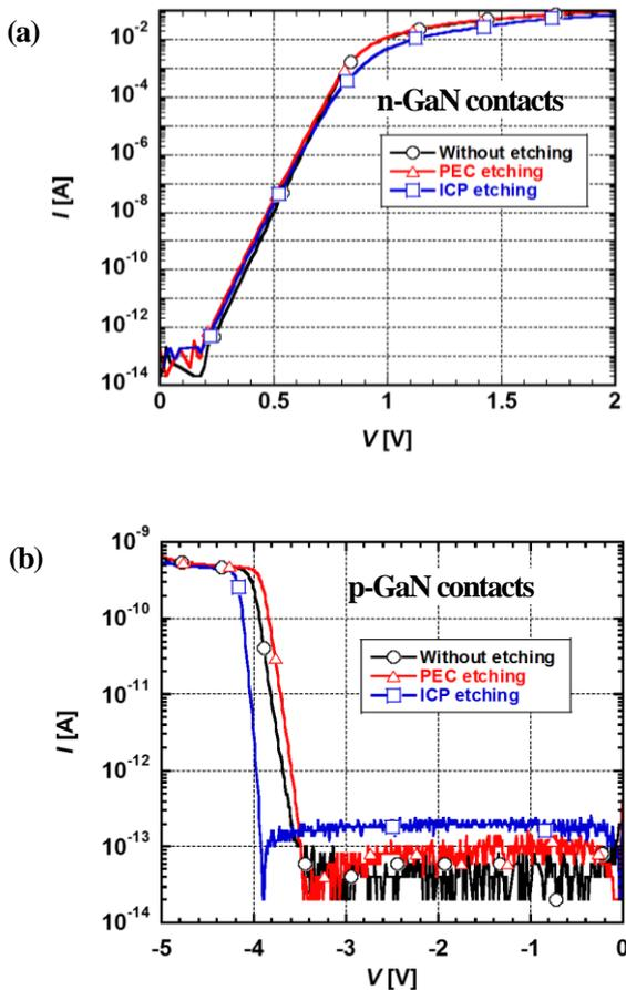
Fig. 2 Forward  $I$ - $V$  characteristics of the (a) Ni/n-GaN, and (b) Ni/p-GaN contacts etched by PEC or ICP etching.
