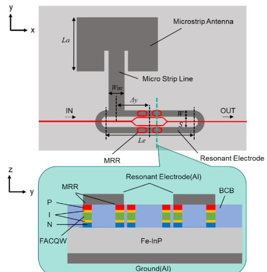
Fig. 1 Schematic view of proposed phase modulator.
