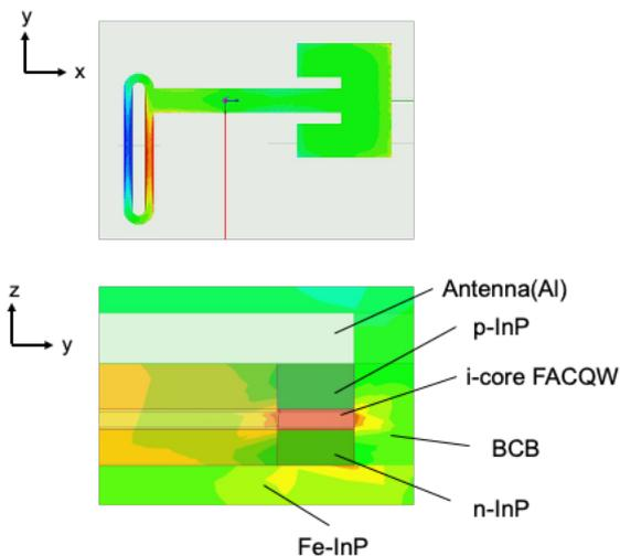
Fig. 2 Calculated distribution of z-component of electric fields  $E_z/E_0$ . (a) Top view. (b) Cross sectional view.
