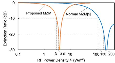
Fig. 4 Modulation characteristics of proposed modulator.
