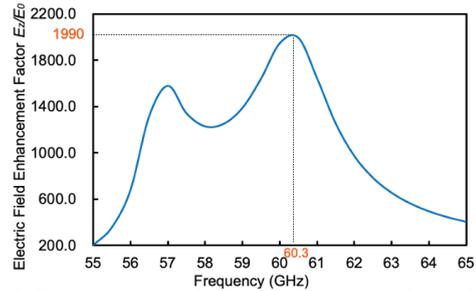
Fig. 3 Calculated electric field enhancement factor  $E_z/E_0$  as function of frequency of MMW plane waves.
