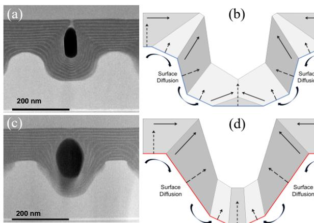
**Figure 1.** TEM images (a and c) and schematics (b and d) illustrating the evolving growth fronts and void formation during regrowth of devices A and B, respectively.
