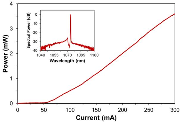
**Figure 2.** Pulsed LI characteristics and lasing spectrum (inset) of device B showing threshold current of 65 mA and emission at 1074 nm.
