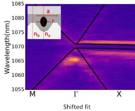
**Figure 3.** Measured and simulated (overlay) band structure of device B. Model used for simulation (inset) constructed from TEM image.
