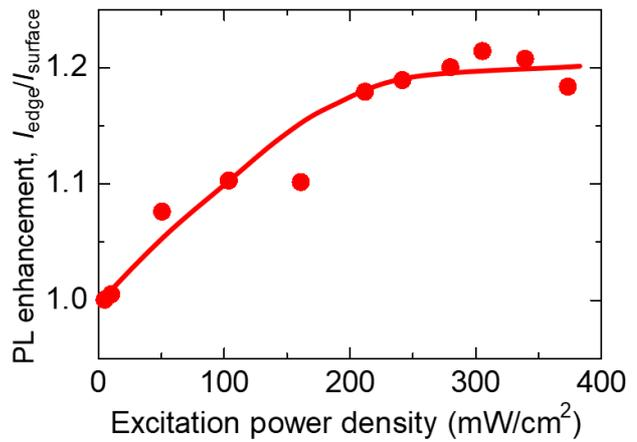
Fig. 4 PL enhancement of Eu emission as a function of excitation power density.
