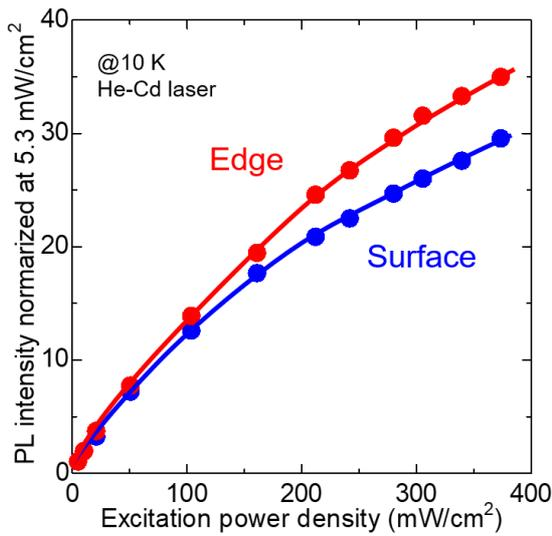
Fig.2 Excitation power density dependences of integrated PL intensities, normalized at 5.3 mW/cm<sup>2</sup>.
