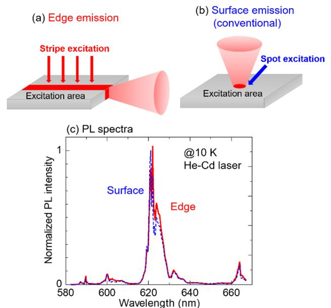
Fig.1 Schematic drawings of PL measurements under (a) EDSE and (b) SDSE configurations. (c) PL spectra from the two configurations at 10 K.
