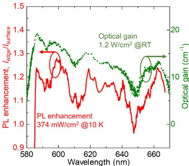
Fig. 3 PL enhancement at 374 mW/cm<sup>2</sup> and net gain as a function of emission wavelength.
