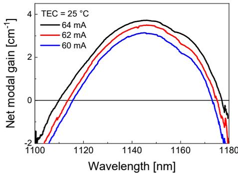
Fig. 3 Gain spectra under various injection currents obtained from the gain chip by the H-P method.
