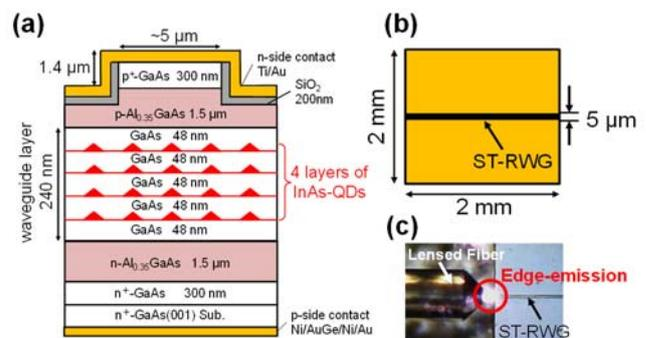
Fig. 1 (a) Schematic profile of a fabricated QD-based gain chip. (b) Illustration of the RWG fabricated on the chip with as-cleaved edges. (c) Photograph of an edge of the RWG coupled to a lensed fiber.
