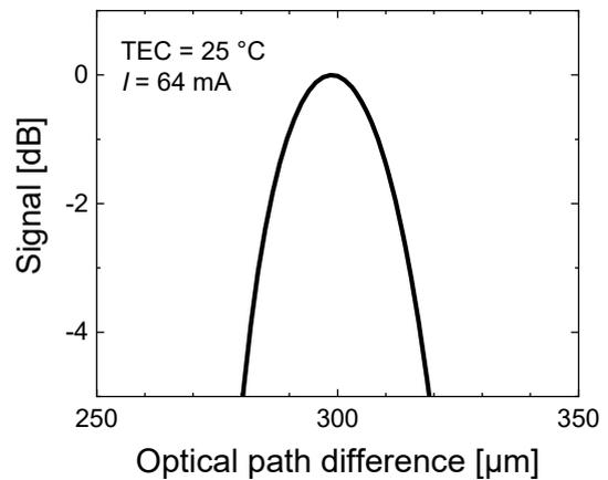
Fig. 5 PSF obtained from the SS-OCT with the tunable laser.
