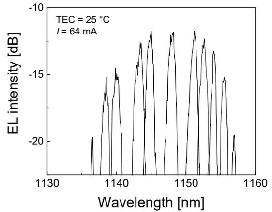
Fig. 4 Tunable lasing spectra obtained from the QD gain chip.
