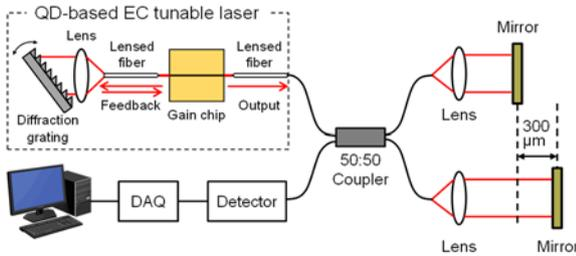
Fig. 2 Schematic of the SS-OCT system with the QD-based EC tunable laser.
