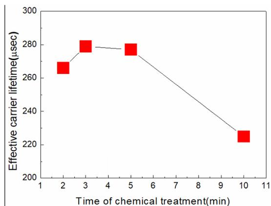
Fig.3. Effective carrier lifetime as a function of time of post-treatment (HCl mixture solution used).
