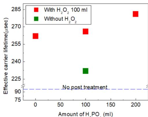
Fig.2. Effective carrier lifetime as a function of oxidizing solution composition (amount of H<sub>3</sub>PO<sub>4</sub> and H<sub>2</sub>O<sub>2</sub>) in chemical treatment
