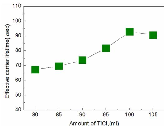
Fig.1. Effective carrier lifetime as a function of amount of TiCl<sub>4</sub> in precursor solution.
