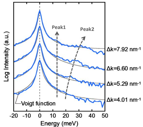
Fig. 1. IXS spectra and Voigt function fitted to the Rayleigh scattering peaks for the  $\text{Si}_{1-x}\text{Ge}_x$  polycrystalline sample measured at different wavenumbers.
