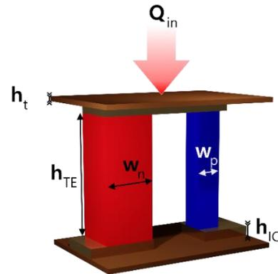
Fig. 1 Schematic of TEG simulated in this work showing parameters.
