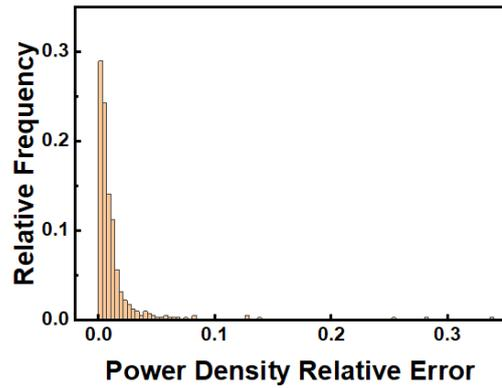
Fig. 4. The distribution of the relative error of the power density for the artificial neural network trained in this work.
