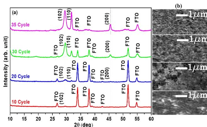
Fig. 1 (a) XRD pattern and (b) SEM view of the sample under cycle conditions for the BiOI/FTO thin films
