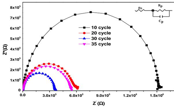
Fig.2 Nyquist plot of the BiOI cells prepared under different SILAR cycle condition
