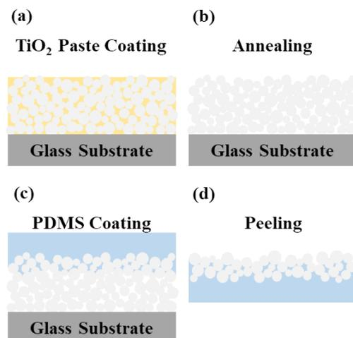
Fig. 1 Fabrication process of the PDMS-TiO<sub>2</sub> composite film. (a) Blade coat TiO<sub>2</sub> paste onto a glass substrate. (b) Anneal the TiO<sub>2</sub> paste. (c) Spin coat PDMS onto the porous TiO<sub>2</sub> layer. (d) Peel off the PDMS-TiO<sub>2</sub> composite film.
