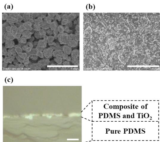
Fig. 2 (a) SEM image of porous TiO<sub>2</sub> nanoparticles on glass substrate after annealed at 370°C. (Scale bar: 1 μm) (b) SEM image of the fabricated PDMS-TiO<sub>2</sub> film showing TiO<sub>2</sub> nanoparticles are randomly embedded on the PDMS surface. (Scale bar: 4 μm) (c) Optical microscopic cross-sectional image of the anti-reflection film. (Scale bar: 5 μm)
