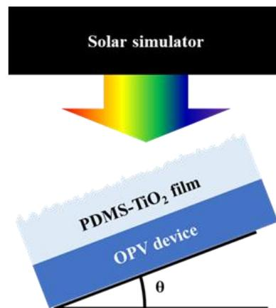
Fig. 3 Experiment setup of measuring the PDMS-TiO<sub>2</sub> film assisted OPV efficiency enhancement at different light incidence angles.
