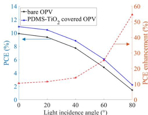
Fig. 4 The OPV efficiency and the enhancement with the PDMS-TiO<sub>2</sub> anti-reflection film at different light incidence angles.
