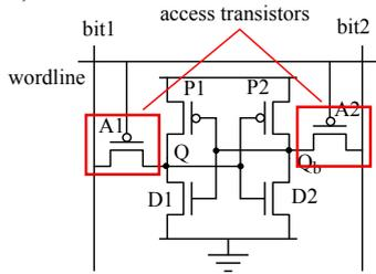
Fig. 1: Circuit schematic of the proposed 6-transistor (6T) SRAM with a pair of p-type access transistors. Compared with the conventional SRAM cell, n-type access transistors are replaced with p-type OTFT.
