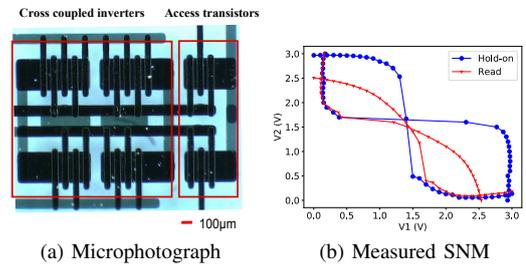
Fig. 6: Test chip microphotograph and the measurements of SNM in hold-on and read states.
