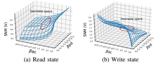
Fig. 4: Simulation results for conventional SRAM structure for finding optimal transistor sizes in read and write SNM at 3V supply voltage.  $\beta_{pd}$  and  $\beta_{ac}$  are swept from 0.4 to 20.
