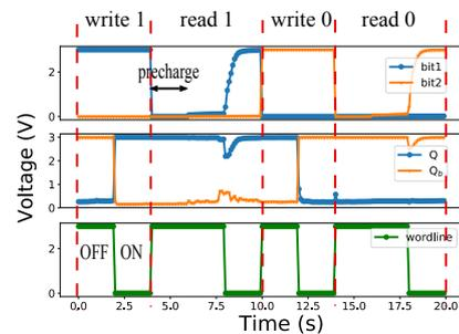
Fig. 7: Write and read operation of the proposed SRAM cell. In each operation, the access transistors are first turned off and then turned on to confirm the operation of the wordline. In read operation, the bitlines are precharged to 0. To confirm read operation clearly, bitlines are connected with 0.1  $\mu$ F capacitors.
