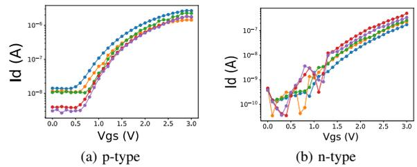
Fig. 5: Measured  $I_d$ - $V_{gs}$  characteristics of OTFTs using the same process with the proposed SRAM.  $L$  and  $W$  of the devices are 50 and 1200  $\mu$ m, respectively.
