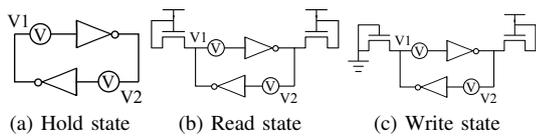
Fig. 2: The test circuits for deriving static noise margin (SNM). SNM is determined by length of the side of the largest square in butterfly diagram drawn by changing V1 and V2.
