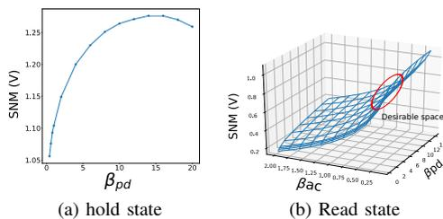
Fig. 3: Optimization of transistor sizes with SNM in hold and read states at 3V supply voltage.  $\beta_{pd}$  is swept from 0.4 to 20 and  $\beta_{ac}$  is swept from 0.2 to 2. Simulation model parameters are based on device measurements in this work.
