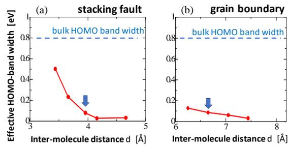
Fig.3 Effective HOMO-band width of the present repeated-slab system in cases of (a) stacking fault and (b) grain boundary, as a function of inter-molecule distance  $d$  around the defect. The arrows indicate the cases of the most stable distances.
