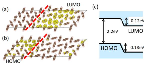
Fig.4 Wave functions of (a) LUMO and (b) HOMO states around the grain boundary. (c) Calculated band alignment around the present grain boundary.
