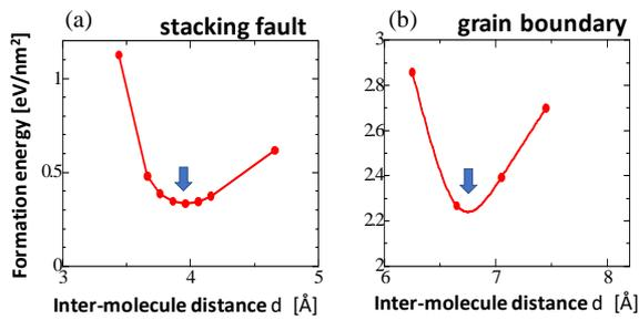
Fig.2 Formation energies of (a) stacking fault and (b) grain boundary, as a function of inter-molecule distance  $d$  around the defect shown in Fig.1. The arrows indicate the most stable distances.
