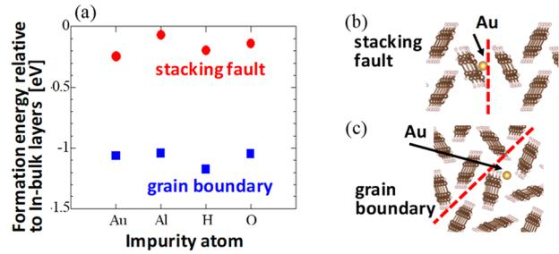
Fig.5 (a) Formation energies of impurity atoms around defects. (b) and (c): Stable Au-atom positions around the stacking-fault and grain boundary.
