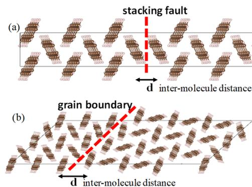
Fig.1 Schematic pictures of (a) stacking fault and (b) grain boundary in pentacene films adopted in the present calculations.
