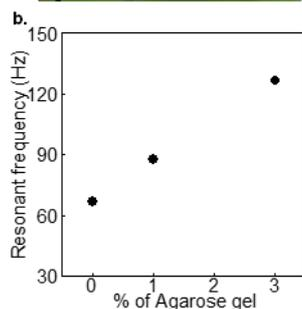
Fig. 3: a. Photograph of in-vitro experimental setup b. Resonant frequency as a function of agarose concentration.
