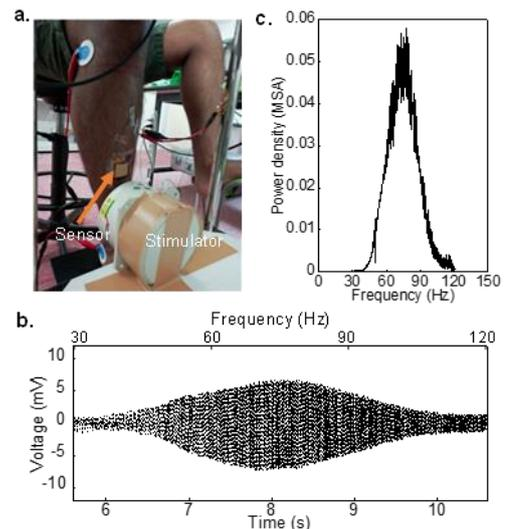
Fig. 1: **a.** Experimental setup for resonance frequency measurement, **b.** Output voltage of sensor when a sweep of 30-120 Hz is applied for 5 s and **c.** corresponding power density.
