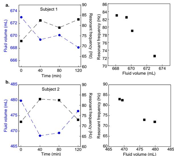
Fig. 4: Shift in resonance frequency due to fluid volume change in a. subject 1 b. subject 2.
