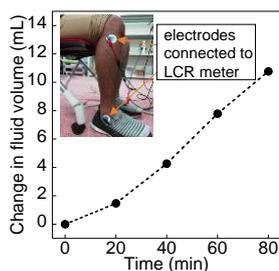
Fig. 2: Fluid volume measurement in lower leg.
