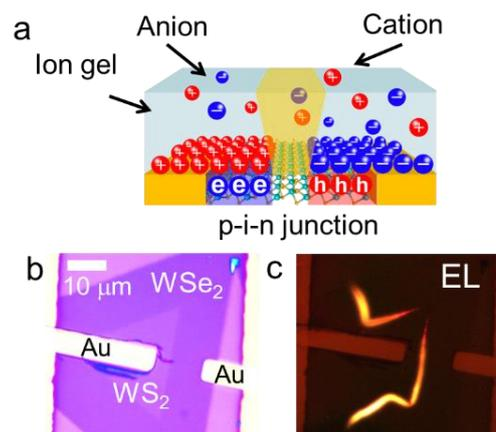
Fig.3 (a) Schematic illustration of the TMDC-based in-plane heterostructure EDLED. (b) Optical and (c) EL images of WS<sub>2</sub>/WSe<sub>2</sub> EDLED device.
