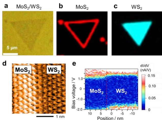
Fig.2 (a) Optical microscopy image, PL intensity maps for (b) 1.77 to 1.94 eV and (c) 1.94 to 2.07 eV, (d) STM image, and (e) color scale map of the dI/dV spectra of a MoS<sub>2</sub>/WS<sub>2</sub> heterostructure.
