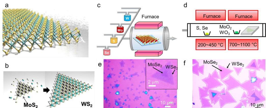
Fig.1 Schematic illustrations of (a) monolayer TMDC and (b) the heteroepitaxial growth of a WS<sub>2</sub>/MoS<sub>2</sub> in-plane heterostructure. (c) Schematic illustrations of CVD systems with (c) liquid precursors and (d) solid precursors. (e) Optical images of WSe<sub>2</sub>/MoSe<sub>2</sub> in-plane heterostructures grown from (e) liquid and (f) solid precursors.
