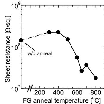
Fig. 6 Sheet resistance of the MoS<sub>2</sub> film underneath the Al<sub>2</sub>O<sub>3</sub> passivation film depending on FG anneal temperature.
