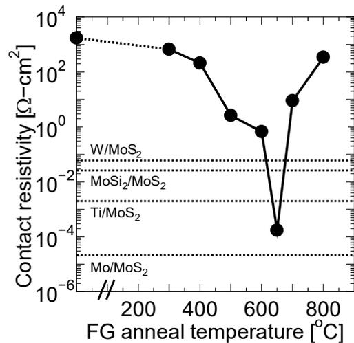
Fig. 7 Contact resistivity at MoS<sub>2</sub>/TiSi<sub>2</sub> interface depending on FG anneal temperature and reported data with various contact metals [5-7,11].
