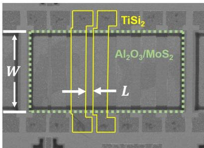
Fig. 3 Top view of the TLM device using sputtered-MoS<sub>2</sub> thin channel with length between contacts of 11-38 μm, width of 247 μm.
