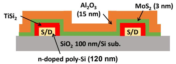
Fig. 2 Cross-sectional schematic image of the MoS<sub>2</sub> channel TLM device structure with the TiSi<sub>2</sub> contact.
