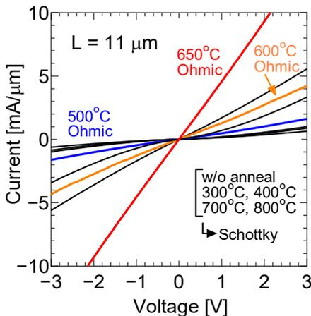
Fig. 4 I-V characteristics at various FG anneal temperatures. Ohmic contacts are observed at 500, 600 and 650°C.
