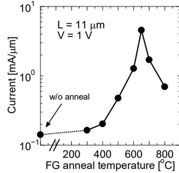
Fig. 5 Current at V=1 V depending on FG anneal temperature. The highest current is observed at 650°C.
