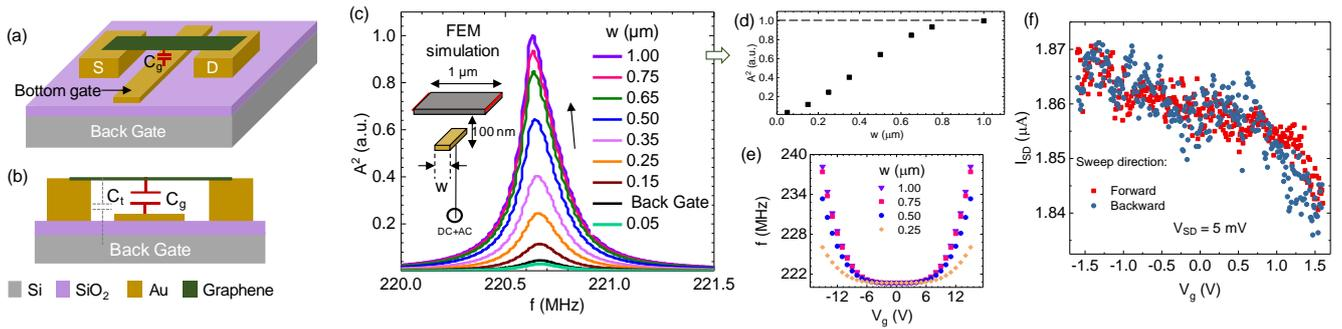
Fig. 1: Schematic illustration of a suspended graphene nano-ribbon with a capacitively coupled local bottom-gate, viewed from (a) side and (top); (c) – (d) Finite-element simulation of electrostatic actuation for different local-gate width ( $w$ ); (e) experimentally acquired ambipolar characteristic in a suspended graphene ribbon indicating capacitive coupling with local bottom gate.
