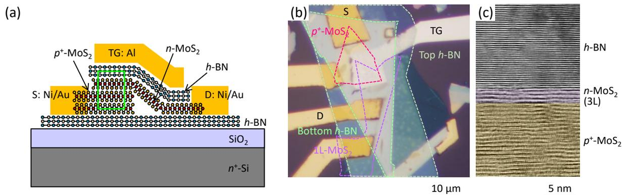
**Figure 1** a) Schematic illustration and b) optical micrograph of all 2D heterostructure TFET. c) Cross sectional TEM image of all 2D heterostructure at the solid rectangular in a). The number of MoS<sub>2</sub> layers is 3.
