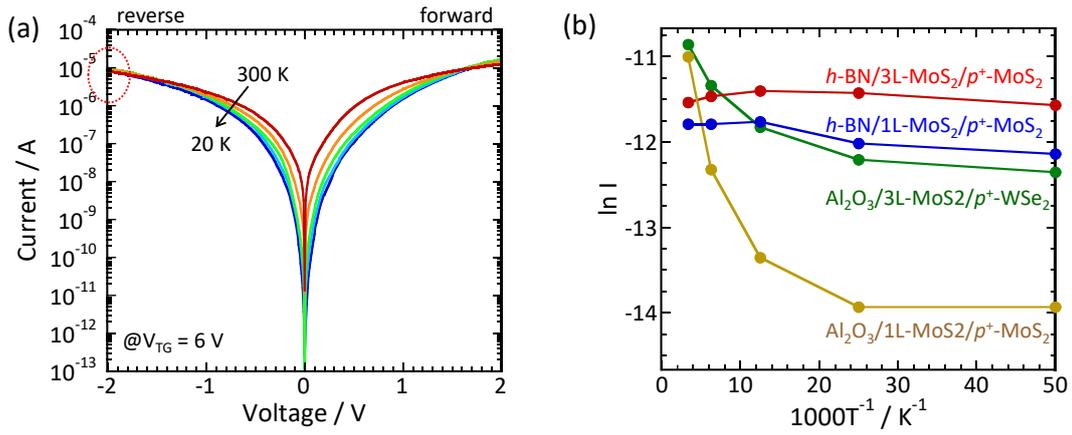
**Figure 2** a) Diode properties in the 3L-*n*-MoS<sub>2</sub>/*p*<sup>+</sup>-WSe<sub>2</sub> heterostructure at  $V_{TG} = 6$  V and different temperatures (20, 40, 80, 160, and 300 K). b) Arrhenius plot of the current at the reverse bias of -2 V for different heterostructures.
