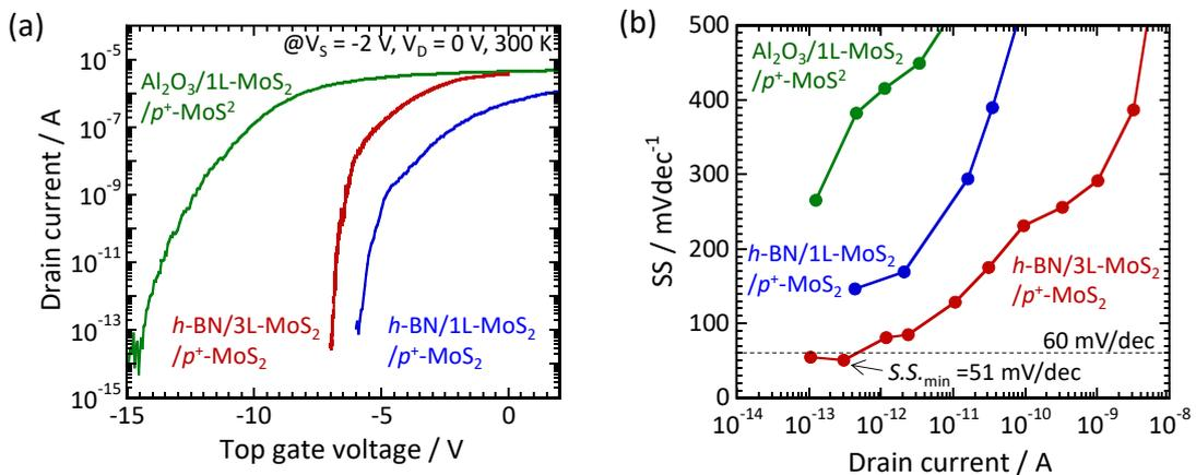
**Figure 1** a) Transfer characteristics for the three different heterostructure TFETs. b) SS as a function of  $I_D$  for the three different heterostructure TFETs.
