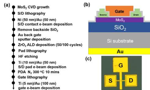
Fig. 1(a) Process flow for fabricating MoS<sub>2</sub> top gate MOSFETs, (b) schematic cross-section and (c) top view of optical microscope photograph of the fabricated devices.
