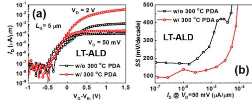
Fig. 5 (a)  $I_D$ - $V_G$  characteristics of 5  $\mu$ m-gate-length 1L MoS<sub>2</sub> top gate MOSFETs measured before and after 300 °C PDA and (b) The  $I_D$  dependence of extracted SS.
