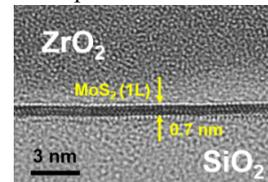
Fig. 2 HR-TEM cross-sectional images of 1L MoS<sub>2</sub> channel with ALD-ZrO<sub>2</sub> gate dielectric.
