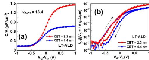
Fig. 6(a) Split-CV characteristics at frequency of 10 kHz and (b)  $I_D$ - $V_G$  hysteresis curves at  $V_D$  of 1 V extracted from 1L MoS<sub>2</sub> devices with different ALD growth cycles.
