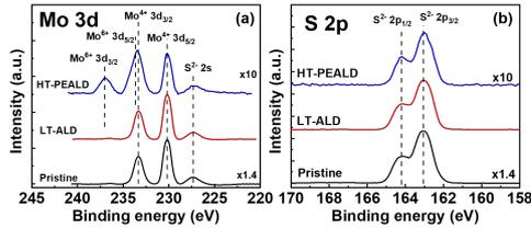
Fig. 3(a) Mo 3d and (b) S 2p XPS spectra extracted from HT-PEALD ZrO<sub>2</sub>/MoS<sub>2</sub>, LT-ALD ZrO<sub>2</sub>/MoS<sub>2</sub> and pristine MoS<sub>2</sub>, respectively.
