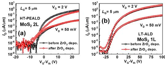
Fig. 4  $I_D$ - $V_G$  transfer curves extracted from MoS<sub>2</sub> MOSFETs under back gate operation before and after (a) HT-PEALD and (b) LT-ALD ZrO<sub>2</sub> encapsulation on top of MoS<sub>2</sub> surface.
