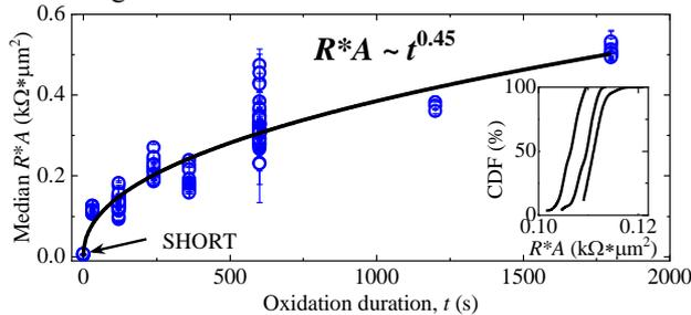
Fig. 3. RA product vs. oxidation duration. Inset: Cumulative distribution for 3 JJ areas from  $t=30\text{s}$  sample with  $\sigma < 2\%$ .
