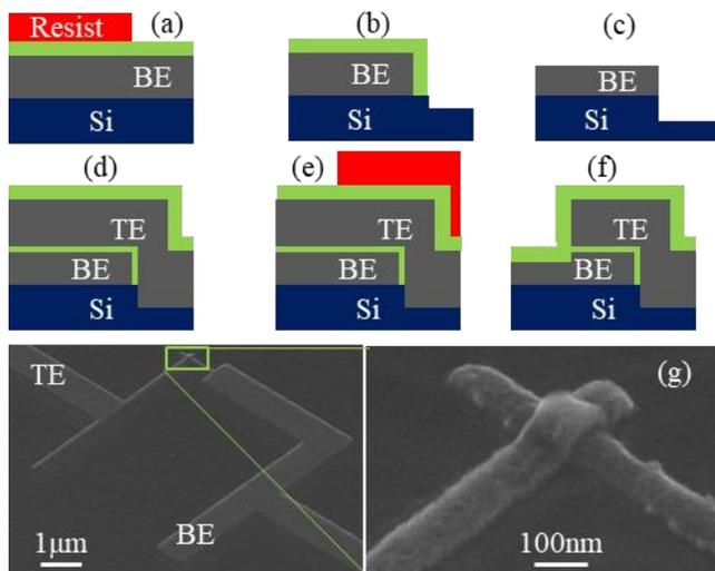
Fig.1. (a) BE deposition and lithography, (b) BE dry etch; (c) Ar sputtering of AlO<sub>x</sub> native oxide (d) in-situ controlled oxidation and TE deposition; (e) TE lithography; (f) final JJ; (g) tilted SEM of a single JJ test structure with nominal area 0.01 μm<sup>2</sup>.
