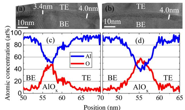
Fig. 2. TEM and elemental profiles (EDS) across JJs formed with (a), (c) 2min and (b), (d) 5 min controlled oxidation.
