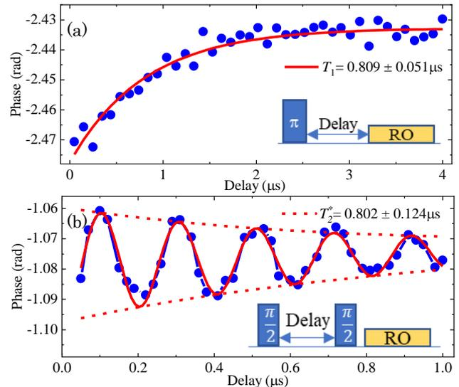
Fig. 4. Qubit relaxation time  $T_1$  (a) and coherence times  $T_2^*$  (b) measurements. The pulse scheme used to perform these characterizations is depicted in the inset.
