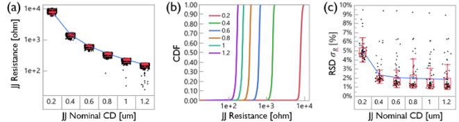
Fig. 5. (a) Resistance, (b) CDF plot, and (c) RSD for all structures.
