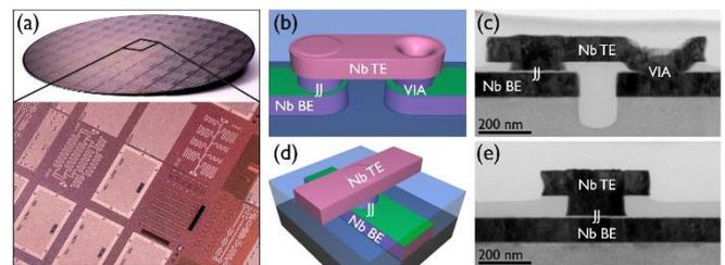
Fig. 2. a) Photograph of a 300 mm wafer with completed trilayer fabrication process, b-c) schematic and TEM cross-section of a JJ and via, d-e) CBKR schematic and TEM cross-section of a single JJ.
