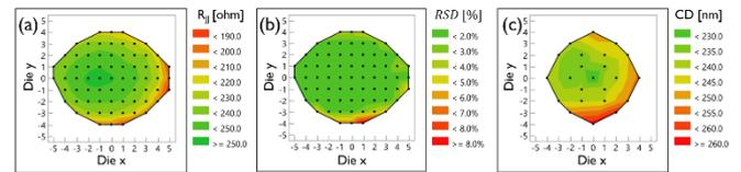
Fig. 6. (a) Resistance wafermap and (b) RSD wafermap for 1 um CD JJ, and (c) CDSEM map for 200 nm JJ
