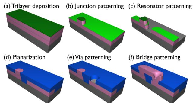
Fig. 1. a-f) Trilayer based superconducting qubit process modules.
