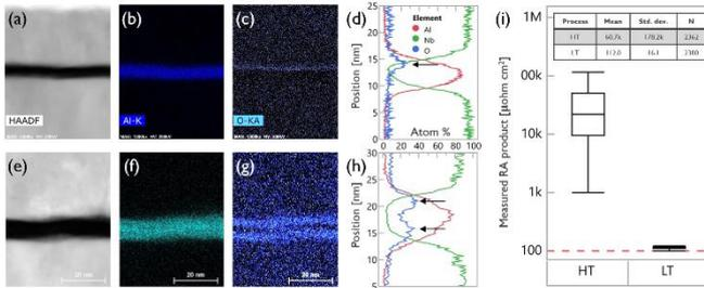
Fig. 3. (a-h) HAADF, EDS, and line scans showing single and double barrier (arrows) for as-deposited and HT trilayers, (i) RA comparison for LT vs HT processes. Red dotted line is the target RA.
