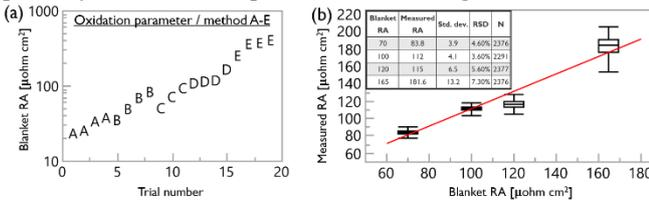
Fig. 4. (a) Blanket RA obtained from CIPT on wafers with varying oxidation parameters and methods, (b) measured RA vs blanket RA. Inset shows  $< 10\%$  variability. The red line is a guide for the eye.
