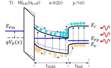
Fig. 4 Schematics to illustrate the operation mechanism of the proposed FED (a) in dark (b) and under UV light illumination. The dashed lines denotes the case without NiO CL.
