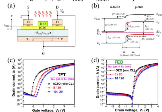
**Fig. 1** (a) Schematic cross section view of the proposed IGZO FED with a patterned NiO CL. (b) The possible energy band diagram of NiO/IGZO HJ under thermal equilibrium. (c) Typical transfer characteristics of the fabricated IGZO TFTs and (d) I–V curves of FEDs without and with NiO CL on the IGZO channel in the dark.
