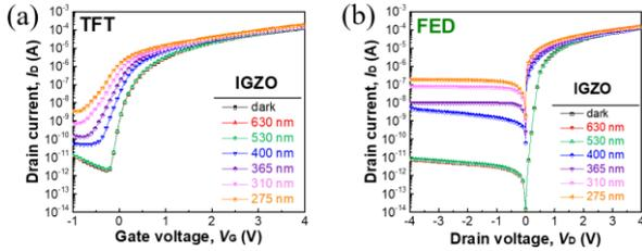
Fig. 2 UV sensing performances of the fabricated (a) TFTs and (b) FEDs.
