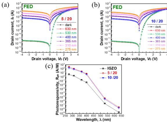
Fig. 3 Experimental  $I - V$  curves of IGZO FEDs. (a) Without NiO CL, (b) with 5- $\mu$ m-wide and 20-nm-thick NiO CL, (c) with 10- $\mu$ m-wide and 20-nm-thick NiO CL, and (d) the corresponding  $R_{ph} - \lambda$  curves.
