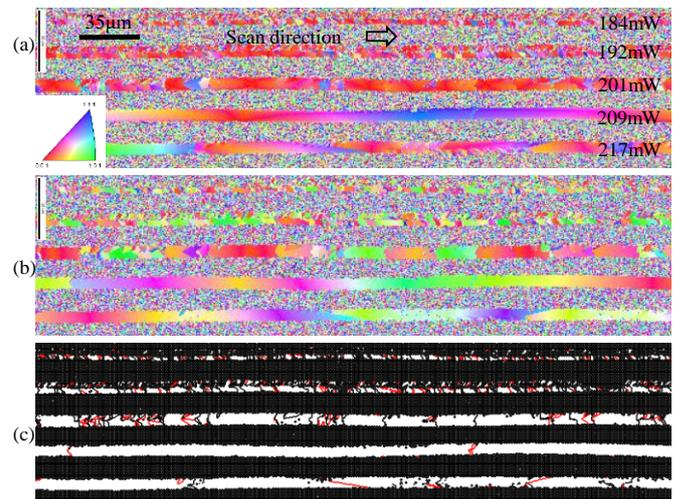
Fig. 1. EBSD crystal orientation map of uncapped Si strip in (a) ND and (b) SD. (c) boundary map
