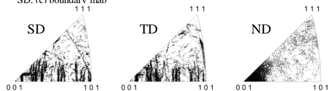
Fig.2 IPF of 1mm-long Si strip at threshold of the lateral growth in SD, TD, and ND
