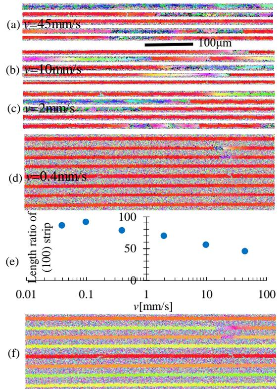
Fig. 5. ND orientation map of Si strip with  $v$  of (a) 45mm/s, (b) 10mm/s, (c) 2mm/s, (d) 0.4mm/s. (e)  $R$  depending on  $v$ . (f) SD orientation map of Si strip with  $v$  of 0.4 mm/s.
