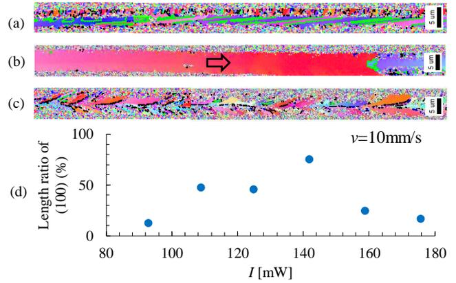
Fig. 4 Typical ND orientation map of Si strip with (a)  $I \leq 93$  mW, (b)  $109 \text{ mW} \leq I \leq 142$  mW, (c)  $I \geq 159$  mW. (d) Estimated length ratio of (100) strip  $R$  depending on  $I$
