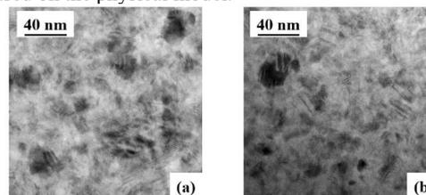
Fig. 6 HRTEM images of solid-phase crystallized a-Si films annealing by  $\mu$ -TPJ at  $v$  of (a) 500 mm/s and (b) 800 mm/s, respectively.
