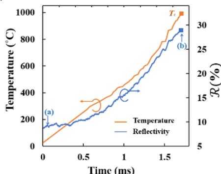
Fig.3. The transient variation of temperature and  $\mathcal{R}$  of a-Si film are extracted from Fig.2(a) to (b).
