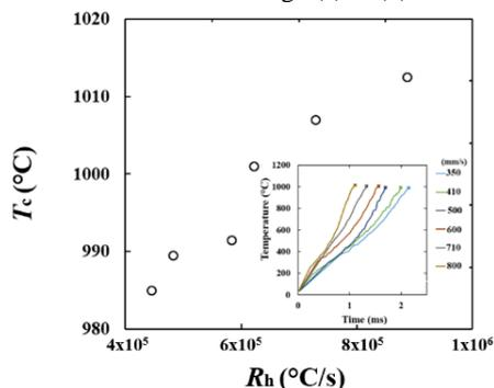
Fig.4. Dependence of  $T_c$  on  $R_h$ . The inset shows the transient variation of a-Si temperature measured under different  $v$  depends on heating time, ■ marks indicate the  $T_c$ .
