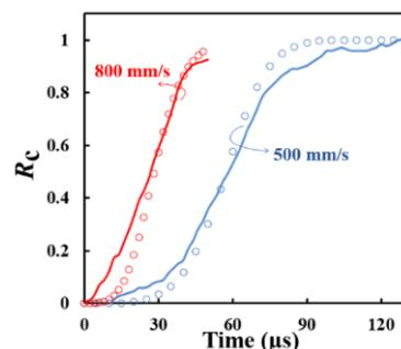
Fig. 5. Crystalline volume fraction as function of time during phase transformation when a-Si film was annealed by  $\mu$ -TPJ under  $v$  as 500 mm/s (a), and 800 mm/s (b), respectively. The dotted line is calculation data of  $R_c$  based on the physical model.
