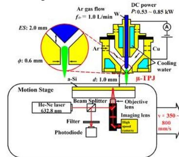
Fig.1. Experimental set-up
