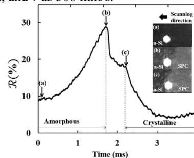
Fig.2. HSC snapshot and transient  $\mathcal{R}$  of 150-nm-thick Si film during  $\mu$ -TPJ irradiation under conditions of  $P = 0.61$  kW,  $d = 1.0$  mm,  $f_{Ar} = 1.0$  L/min, and  $v = 500$  mm/s.
