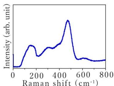
Fig. 2 Raman spectrum of printed Si film annealed at 400°C
