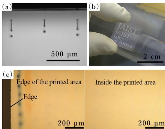
Fig. 1 Inkjet printing of liq-Si. (a) Inkjet droplets discharging from three nozzles. (b) printed Si pattern on substrate. (c) Micrographs of the printed area at edge and inside.
