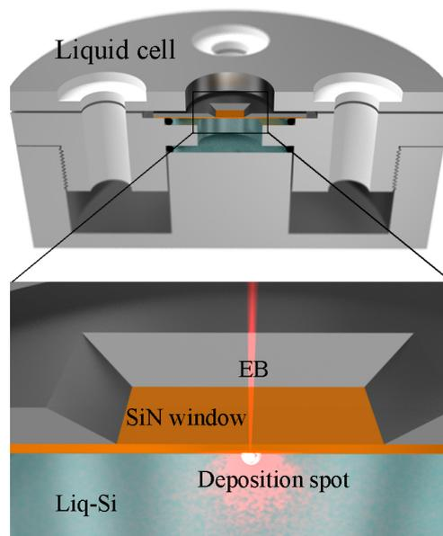
**Figure 1.** Liquid-phase electron beam induced deposition (LP-EBID) of liq-Si. The schematics of liquid cell and EB irradiation.
