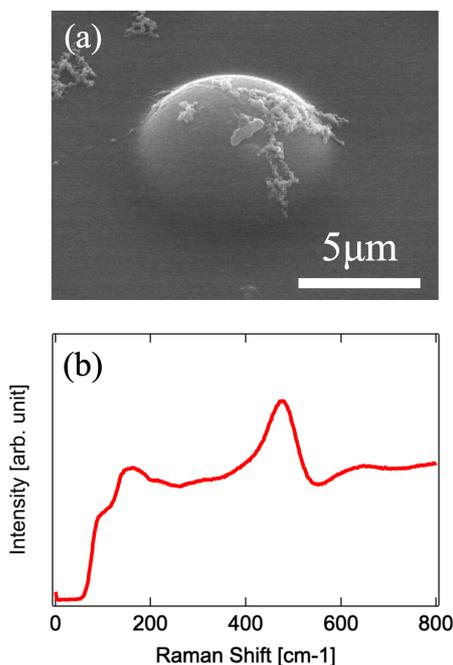
**Figure 3.** The deposit obtained by giving sufficient doses. (a) Scanning electron micrograph of bird's eye view (b) Raman spectrum.
