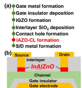
Fig. 5 (a) Fabrication process and (b) schematic image of IGZO-FET w/ IAZO-CL.
