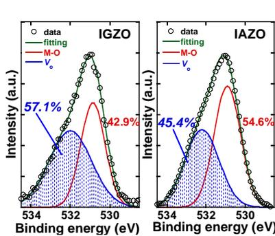
Fig. 3 XPS spectra of O1s in IGZO and IAZO film. The peak area of  $V_O$  in IAZO film is smaller than that in IGZO film.
