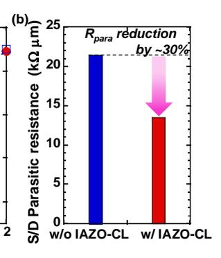
Fig. 7 (a)  $R_{on}$ - $L_g$  plot and (b) comparison of  $R_{para}$  between IGZO-FET w/ and w/o IAZO-CL.  $R_{para}$  is decreased by 30% by the insertion of IAZO-CL.
