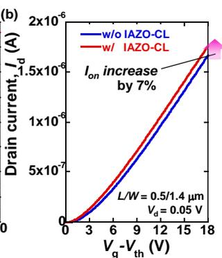
Fig. 6  $I_d$ - $V_g$  characteristics of IGZO-FET w/ and w/o IAZO-CL after annealing at  $420^{\circ}C$  under  $N_2$  atmosphere. Drain current of IGZO FET w/ IAZO-CL was increased by 7%.
