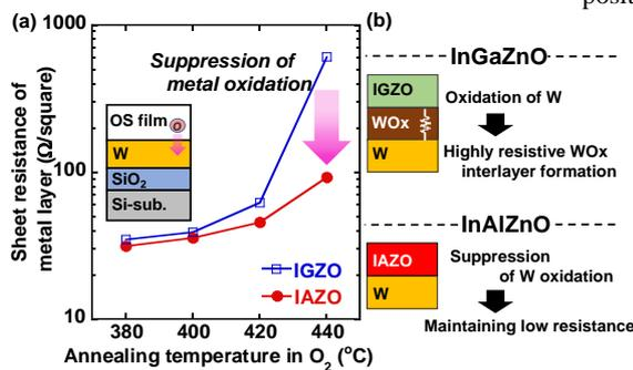
Fig. 4 (a) Annealing temperature dependence of sheet resistance of tungsten film covered by OS materials and (b) schematic diagram of comparison between IGZO and IAZO.
