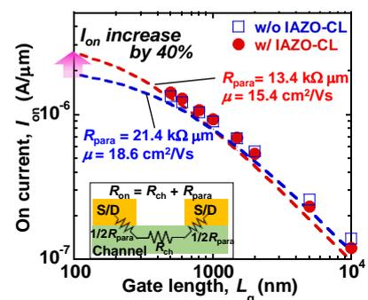
Fig. 10  $I_{on}$  improvement by  $L_g$  scaling calculated from extracted mobility and  $R_{para}$ .  $I_{on}$  is expected to increase by 40% with IAZO-CL at  $L_g = 100$  nm.
