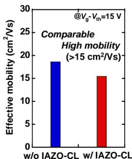
Fig. 8 Effective mobility extracted by split C-V method. High mobility (>15  $cm^2/Vs$ ) was maintained.
