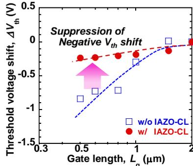
Fig. 9  $\Delta V_{th}$  roll-off curve after annealing at  $420^{\circ}C$  under  $N_2$  atmosphere. Negative shift of  $V_{th}$  was reduced by insertion of IAZO-CL.
