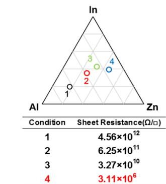
Fig. 2 Chemical composition and sheet resistance of deposited IAZO films. IAZO film with less Al composition shows a lower resistivity.
