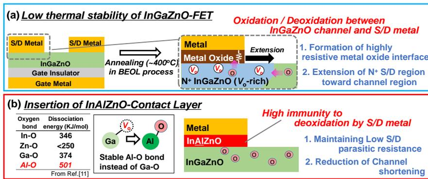
Fig. 1 (a) Schematic illustration of issues in IGZO-channel FET for high-temperature annealing, and (b) list of metal-oxygen bond dissociation energy [11] and concepts of a reduction of S/D parasitic resistance and a suppression of channel shortening by IAZO-contact layer.
