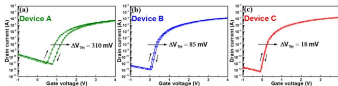
**Fig. 4** Hysteresis loops of (a) device A, (b) device B, and (c) device C under the forward (-1 to 4 V) and reverse (4 to -1 V) sweeps.
