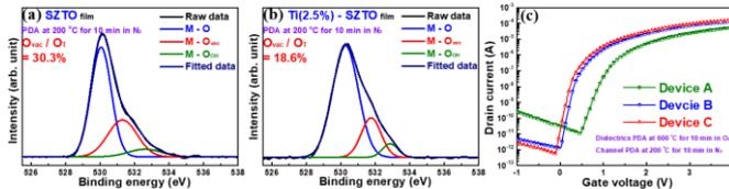
**Fig. 3** O 1s core-levels XPS spectra of (a) SZTO and (b) Ti(2.5%)-SZTO (c) transfer characteristics of devices A, B, and C.
