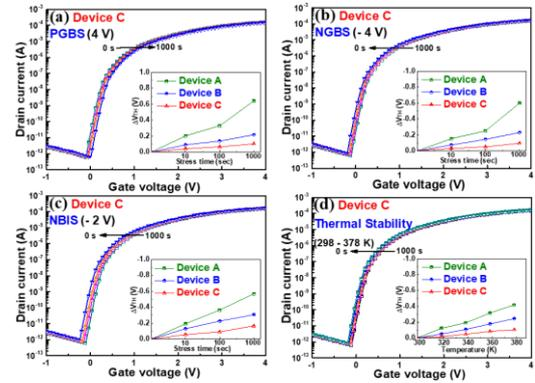
**Fig. 5** The transfer characteristics of device C under (a) PGBS, (b) NGBS, (c) NBIS, and (d) thermal stability tests. The inset in these figure shows the measured  $\Delta V_{TH}$  as a function of stress time for devices A, B, and C.
