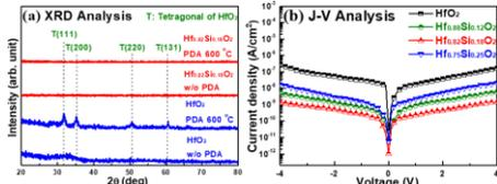
**Fig. 2** XRD analysis of  $\text{HfO}_2$  and  $\text{Hf}_{1-x}\text{Si}_x\text{O}_2$  films without and with PDA at  $600 \text{ }^\circ\text{C}$  for 10 min in  $\text{O}_2$  ambient. (b) J-V curve of MIM capacitors with  $\text{HfO}_2$  and  $\text{Hf}_{1-x}\text{Si}_x\text{O}_2$  dielectrics after PDA at  $600 \text{ }^\circ\text{C}$  for 10 min in  $\text{O}_2$  ambient.
